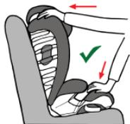
*NOTE: Even with UAS properly attached and adjusted, child seat will still have movement against the vehicle seat back and bottom.*
